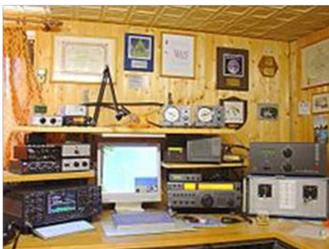
Fig 1. An example of an amateur radio station with four transceivers, amplifiers, and a computer for logging and for digital modes.
